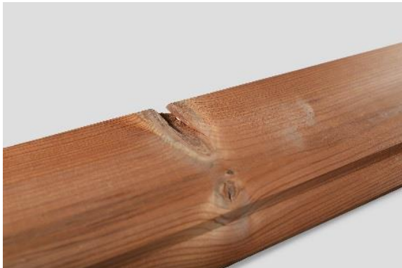
Large crack of a (sound) knot.
